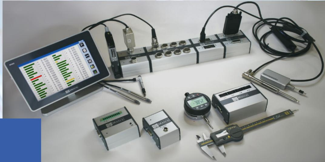
« The M-Bus network can be used to connect probes and measuring instruments of different brands to Metro displays, a PLC or a PC.»
