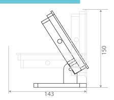
The case is made of machined aluminium and comes on a swivel base that can be fixed using 4 M5 threads.
