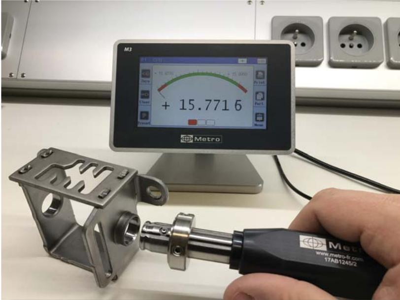
16N7 Internal diameter measurement on a air plug gage directly connected on a M3 display
