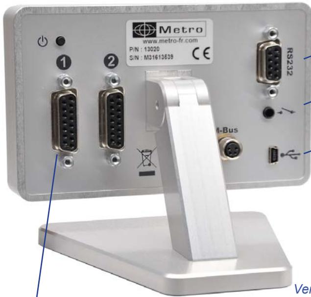
RS232 with ASCII protocol or modbus RTU
