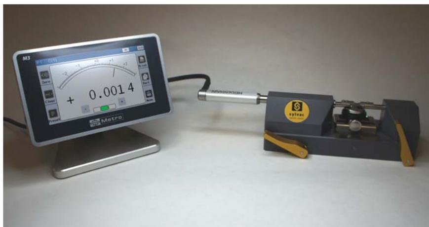
Measurement of very small watch parts. Here the M2 is connected with a Heidenhain SPECTO probe, mounted on a Sylvac PS15 measuring bench.
