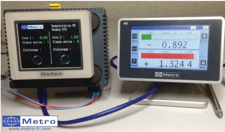
Communication between a M3 display and a Proface PLC with the Modbus RTU protocol. The HMI from Proface has been programmed with different buttons and indicators allowing to control and bring back information from the M3.
